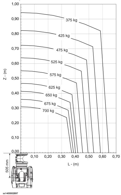
1.5.3 Maximum load and moment of inertia for full and limited axis 5 (center line down) movement
